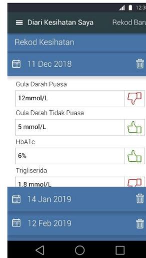
Figure 3 Examples of WeSihat application interfaces that are designed with large button size and spacing, minimizing the use of keyboard and using drag and pinch movement.
