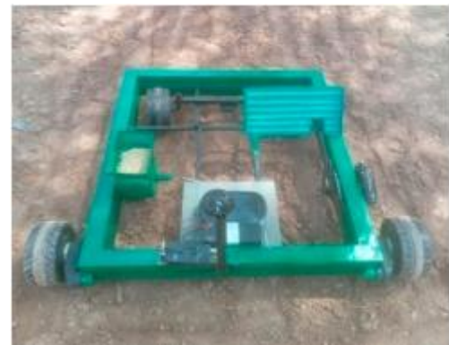
Figure 1.2 Fabricated Model of Seedling and Seed Sowing Robot
