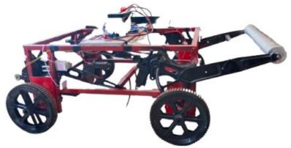
Figure 1.1 Fabricated Model of Plowing and Leveling Robot
