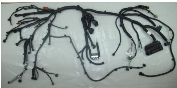
Fig. 1: Example of Electrical Engine Harness
