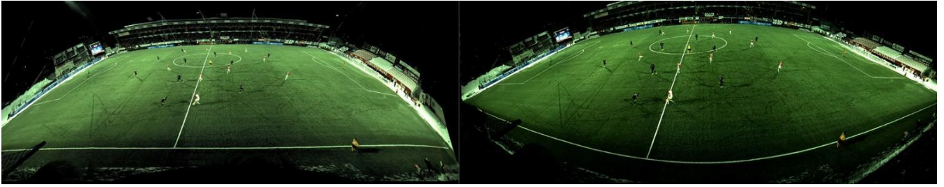
Figure 5: Example of distortion correction for ultra-wide real-time video. Corrected video (left) and original Video (right).
