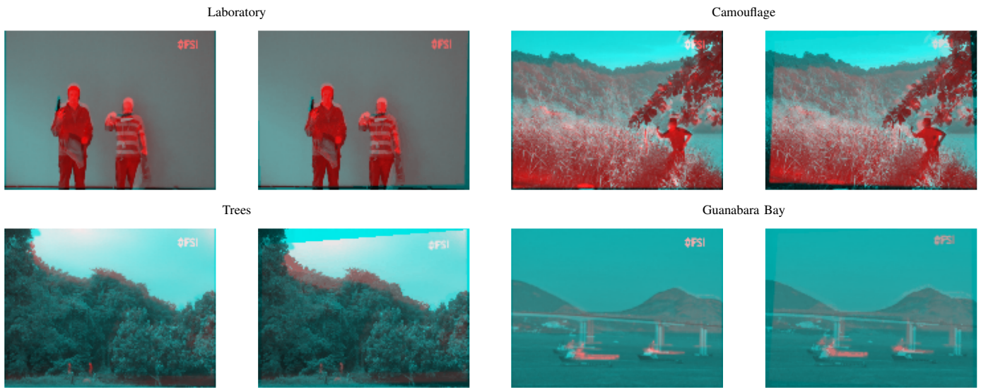
Fig. 3. For each scene, thermal-visible fusion without registration (left), with the proposed registration (right).
