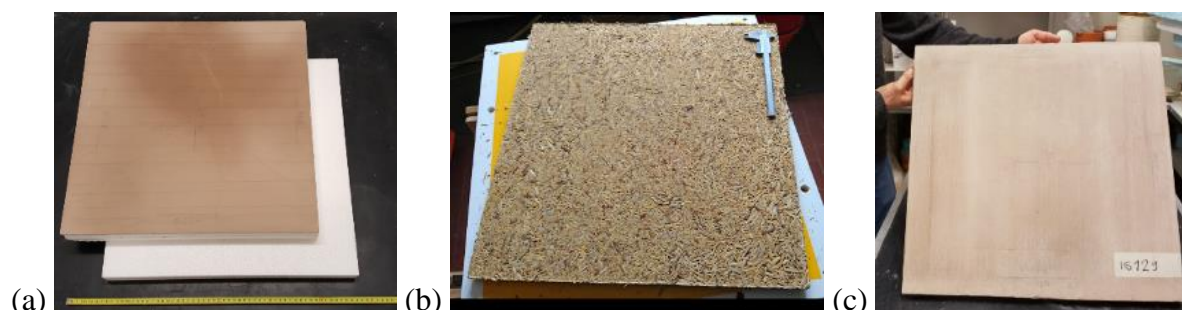
Figure 1: InnoWEE products. a) ETICS-like panel prototype 50×50 cm with 8 cm thick EPS, (b) WGP 60×60 cm and 15 mm thick for backside reinforcement of ventilated façade panels, (c) ventilated façade panel.
