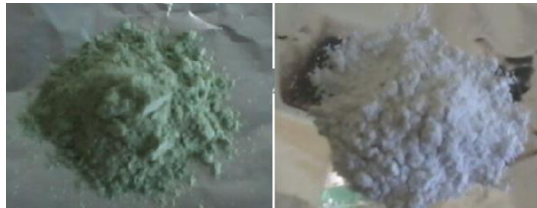
Fig. 3. Picture of of the two nano-materials SrMP 2 O 7 (M = Gd or Ce) at 1000 °C.
