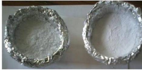
Fig. 1. Picture of the two nano-materials SrMP 2 O 7 (M = Gd or Ce) inside the alumina crucible at 25 °C.
