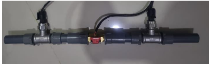
Figure 2. 6 Liquid Flow Sensor and Liquid pressure sensor design
