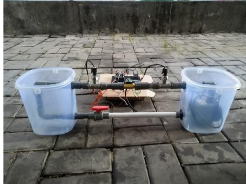
Fig 2. 4 Plant Simulator Fluid Measuring System
