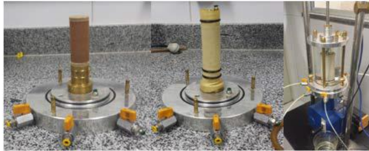
Fig. 15. Set-up of specimen in triaxial apparatus
