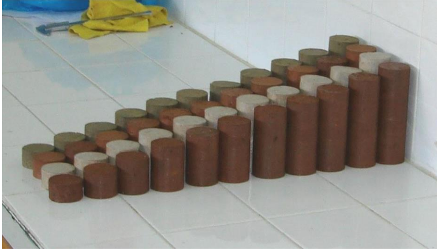
Fig. 20. Photograph of the specimens used in the UCS tests (from left to right: Handere clay, Almanpinarı clay, kaolinite, and Sam-Tekin clay)
