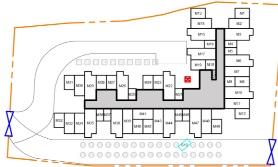
Figure 7: Layout with minimum lifting moment ( \theta_S = 40^\circ )
